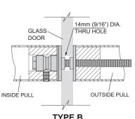
TYPE B (PLASTIC WASHER WITH STEP BUSHING)
