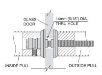
TYPE B (PLASTIC WASHER WITH STEP BUSHING)
