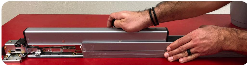
**12. FLIP OVER RE-INSTALL (4) SCREWS TO SECURE BASERAIL TO HOUSING.**
