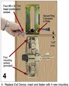
screws (do not over-tighten). Before mounting the Battery Box Mounting Plate, carefully pull wires from door through center of Plate. Do not pinch or cut wires. Position the Plate a minimum of 1/4" **above** Exit Device. Fasten the Battery Box Mounting Plate with four #8 x 3/4" flat head combination screws, using one of the screws to secure the green ground wire ring connector to the Plate.
