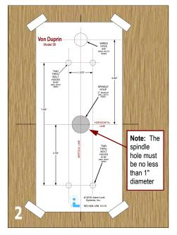
2. Existing Installation: Position Alarm Lock template on horizontal & vertical lines of existing spindle hole.
