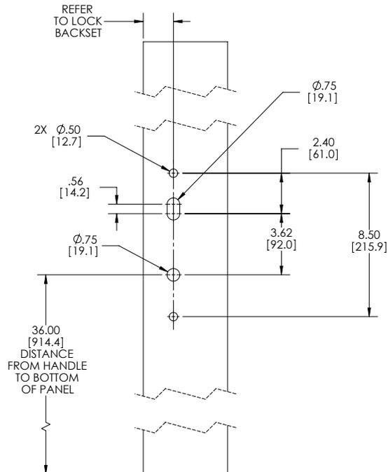
**FIG. 6 SENTRY HINGED PATIO DOOR HANDLE SET, SEMI-ACTIVE ASSEMBLY**
