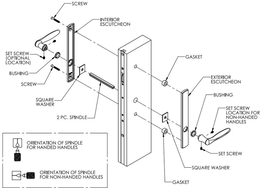
FIG. 9 SENTRY HINGED PATIO DOOR HANDLE SET, PASSIVE DOOR PREPARATION
