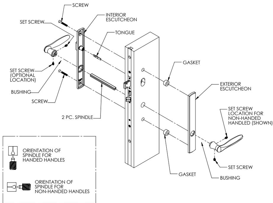
**FIG. 7 SENTRY HINGED PATIO DOOR HANDLE SET, SEMI-ACTIVE DOOR PREPARATION**
