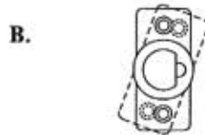
B. Rotate latch face clockwise 20° and pull out latch face.
