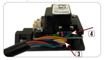
Using double sided tape, secure MM4S to inside of the back of exit device housing. Connect Molex Pigtail. Add Mounting Pad & cable tie to secure cable wires.
