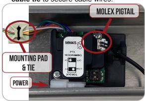
11. Connect to Power & Set the "Push to Set Adjustment" following the steps below.
